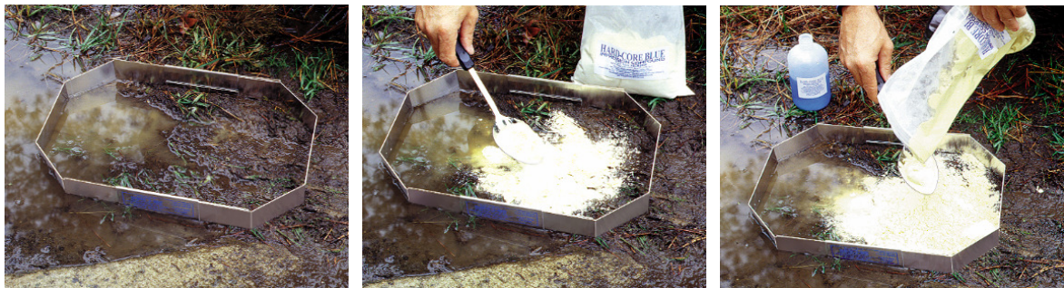
plaster cast mixes - application
